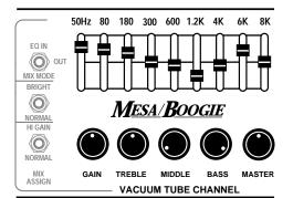
Select the VACUUM TUBE CHANNEL using the footswitch labeled TUBE on the Foot Controller and set the controls as per this example.
